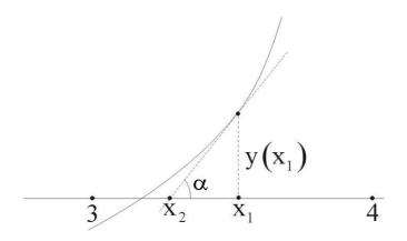
The first step is to find  $x_2$ . Here is the description of the Newton Method:
